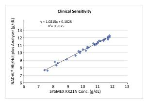
As the results show, all tested samples were almost consistent with the expected haemoglobin concentration. The clinical sensitivity of the NADAL® Hb/Hct plus Analyser is 95%. The correlation coefficient (R<sup>2</sup>) is 0.9875.
