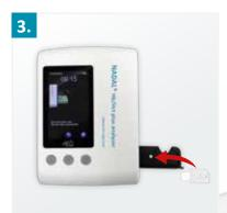
Place the microcuvette with the sample into the holder and close it fully. The test will begin automatically.
