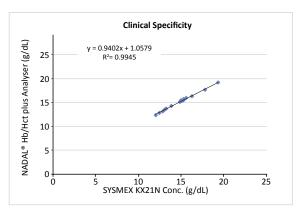
As the results show, all tested samples were almost consistent with the expected haemoglobin concentration. The clinical specificity of the NADAL® Hb/Hct plus Analysers is >99.99 %. The correlation coefficient (R<sup>2</sup>) is 0.9945.
