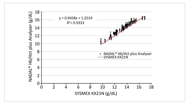
The NADAL® Hb/Hct plus Analyser demonstrates good correlation with the Sysmex KX21, with a correlation coefficient of 0.9333.
