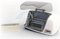
Up to 24 identical or completely different strips can be loaded on the moving arm.
