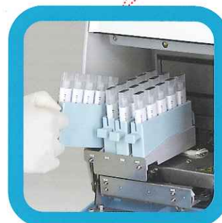
Continuous loading samples, latex reagent and buffer is available during analysis.
