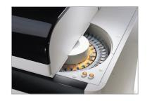
Covered system The pipetting system is covered to ensure safety. The sample disk is flexible to be partially covered only allowing convenient access
