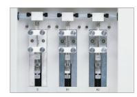
• High pipetting precision 15~300 μL reagent with step at 0.5  $\mu$ L, 1.5~35  $\mu$ L sample with a step at 0.1  $\mu$ L.
