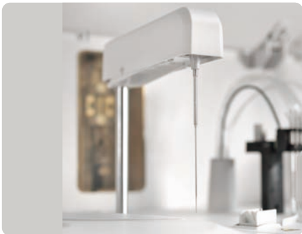
Intelligent probe with optional clog detection
