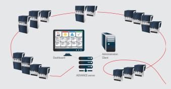
The BOND-ADVANCE network removes traditional IHC limits. With a powerful central network server, BOND-ADVANCE lets you deploy up to thirty BOND instruments on a single unified network.
